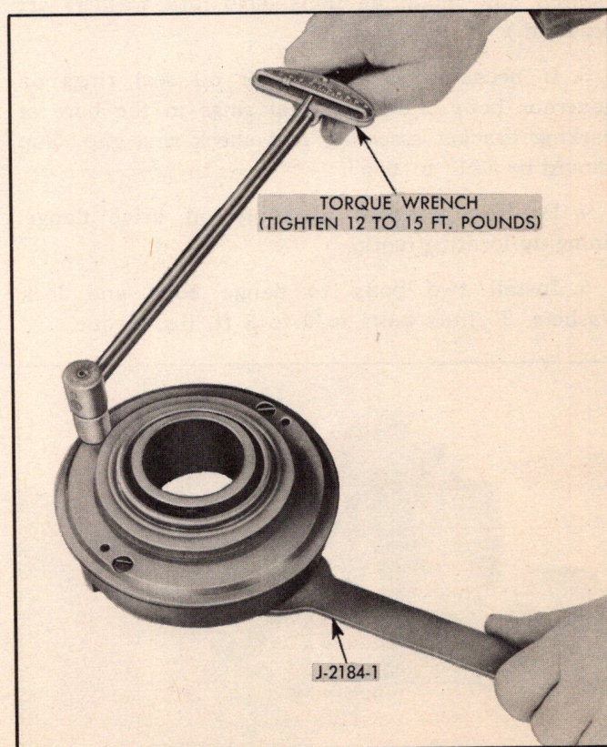
Fig. 278—Installing Pump Cover
