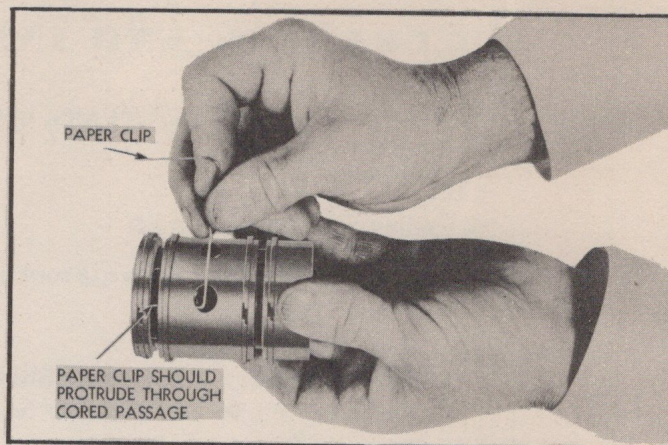
Fig. 189—Inspecting Passages in Oil Delivery Sleeve
