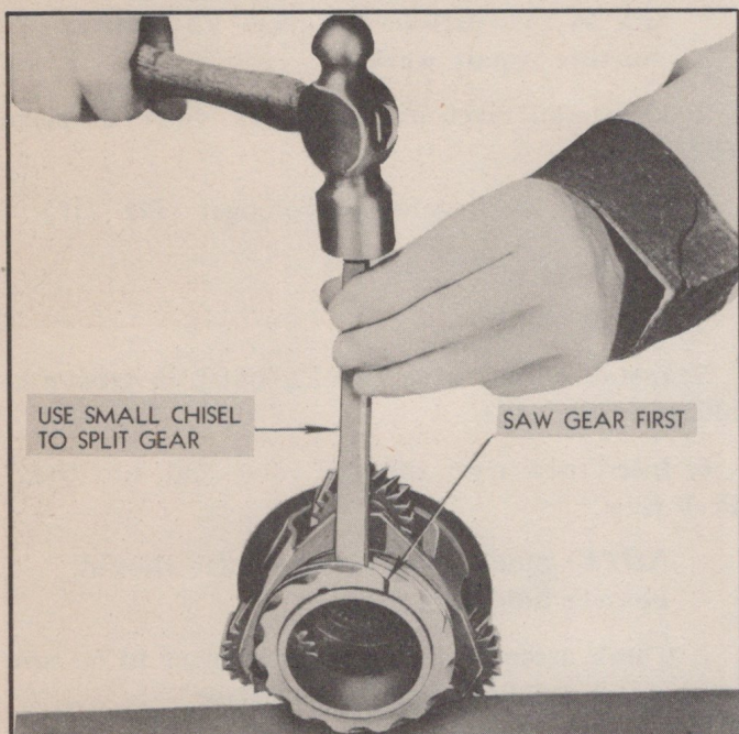
Fig. 220—Removing Oil Pump and Governor Drive Gear
