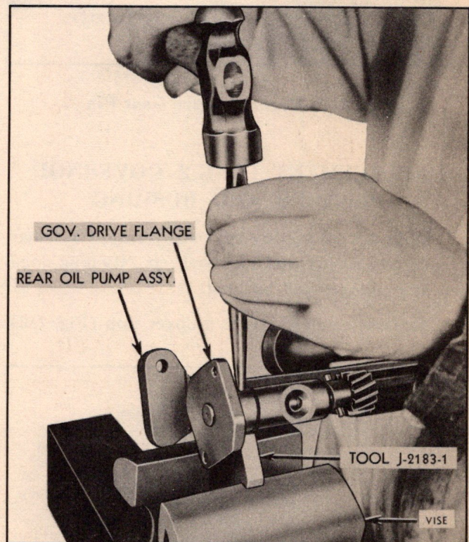
Fig. 211—Removing Governor Drive Flange
