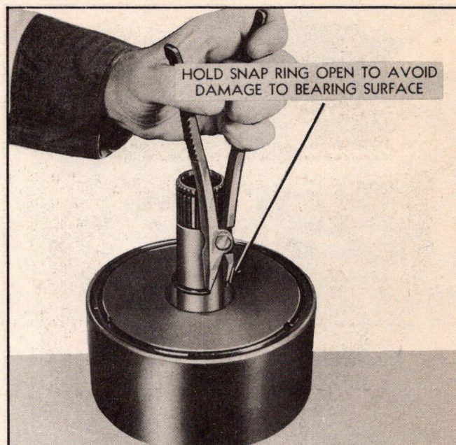
Fig. 134—Removing Snap Ring from Recess in Front Unit
